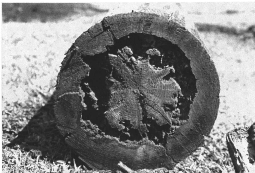
Figure 2. Creosoted telephone pole hollowed out by Formosan termites.
