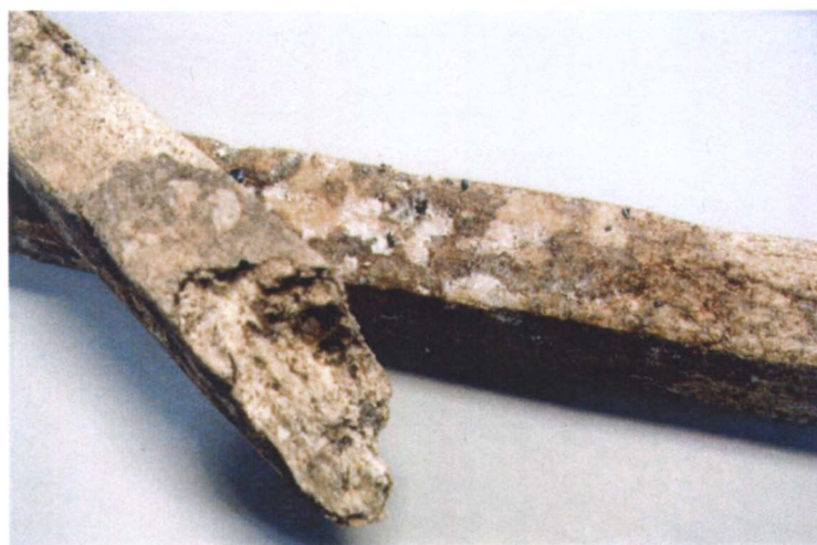
Figure 29.5. Failure break of a WPC field stake after exposure in-ground for 3 years in Saucier, Mississippi.
