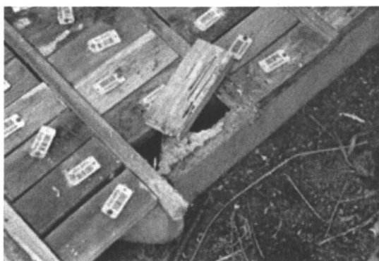
Figure 4. Ground proximity termite field test.
