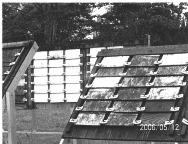
Figure 5. Aspen siding specimens exposed at 45° (foreground) and 90° (background) near Hilo, HI. The 45° exposure angle provides accelerated durability data compared to the 90° exposure (see Figure 6). The specimens shown have similar preservative treatments and have been exposed for the same time interval. Photo by G.M. Larkin
