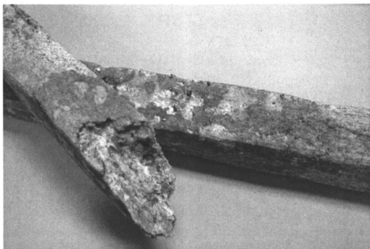
Figure 5. Failure break of a WPC field stake after exposure in-ground for 3 years in Saucier, Mississippi. (See page 10 of color inserts.)
